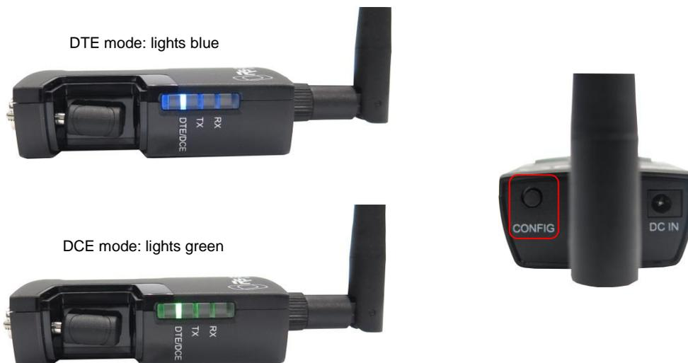
Press the CONFIG button in 3~5 seconds, the TX LED indicator (Orange) starts blinking and go next step for configuration.
