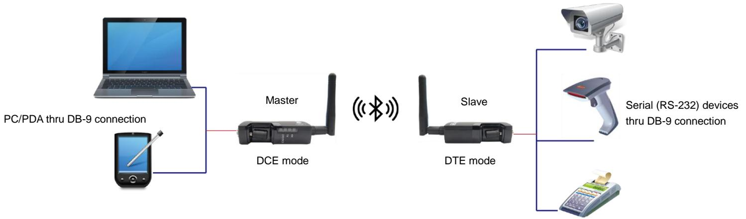
2 BT RS-232 dongles set as DCE/DTE mode are installed between a PC or PDA (Master) and serial (RS-232) devices by DB-9 connections.
